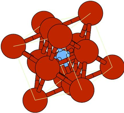
Fig. 1. Geometry of the crystal of  $\gamma$ -Fe<sub>4</sub>N. The Wyckoff positions of the atoms are 1b for nitrogen, and 1a and 3c for the iron. The nitrogen is effectively a body-centered interstitial in the face centered cubic system.
