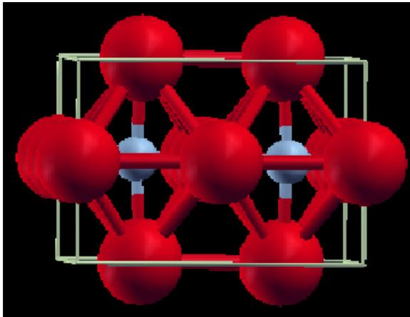
FIG. 3. Low symmetry Fe<sub>4</sub>N Unit cell at 10 GPa with space group P2/m
