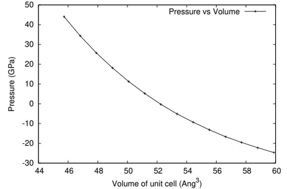
FIG. 2. Variation of the Pressure of  $\gamma' Fe_4N$  crystal as a function of volume
