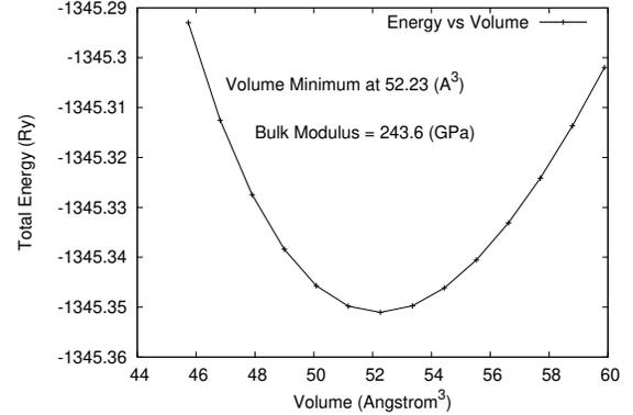
FIG. 1. Variation of the total energy of  $\gamma^{prime} Fe_4N$  crystal as a function of volume
