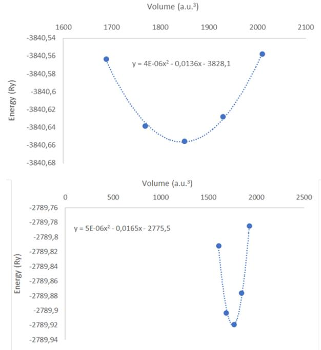
FIG. 4. Energy vs volume for Nb (top) and W (bottom)
