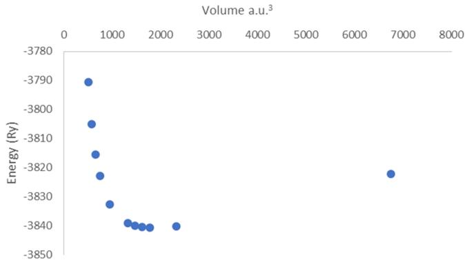
FIG. 3. Energy versus volume for Nb as center atom
