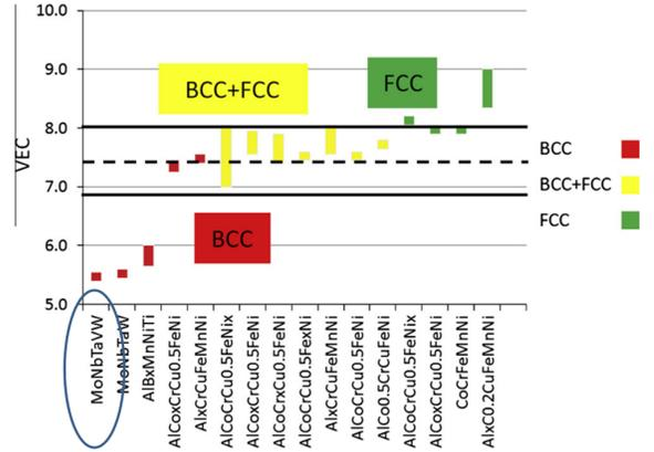
FIG. 1. Different high entropy alloys and their possible unit lattices
